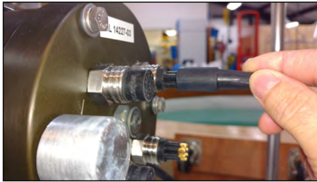
Figure 4-6: Connecting the COM Cable
