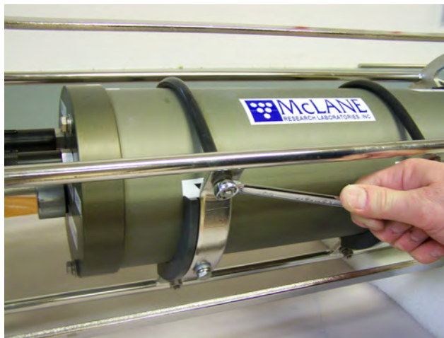
Figure A.3-10: Loosening U-Bolt Clamp
