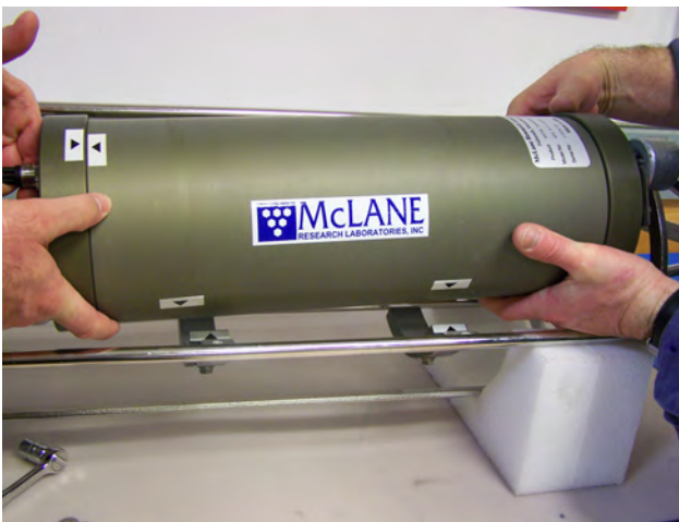
Figure A.3-14: Returning Controller to Frame Figure A.3-15: Aligning Arrows, Reattaching Connector
