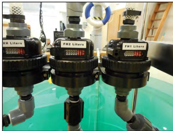
Figure A.1.3-11: Mechanical Flow Meters
