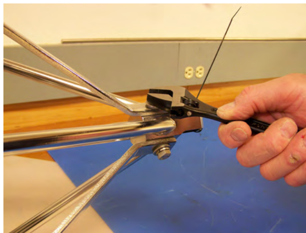
Figure A.3-8: Loosening Frame Guard
