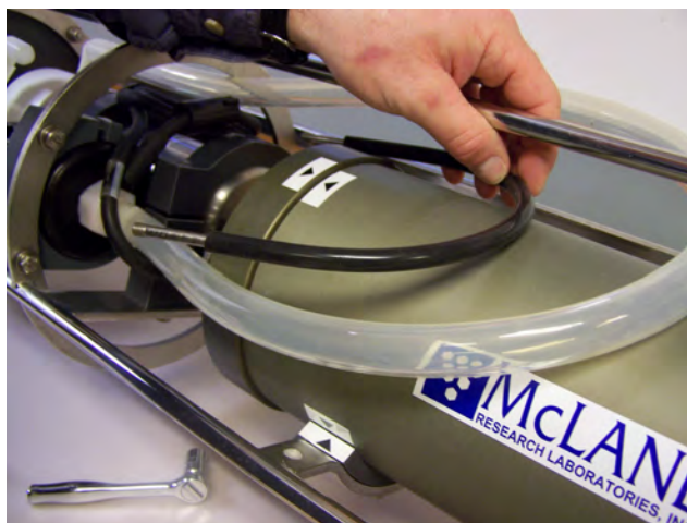
Figure A.3-11: Removing U-Bolt
