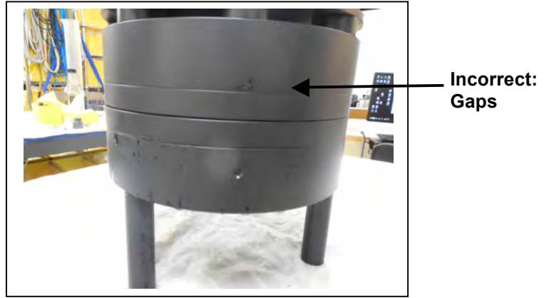
Figure 6-13: Incorrectly Closed Filter Holder
