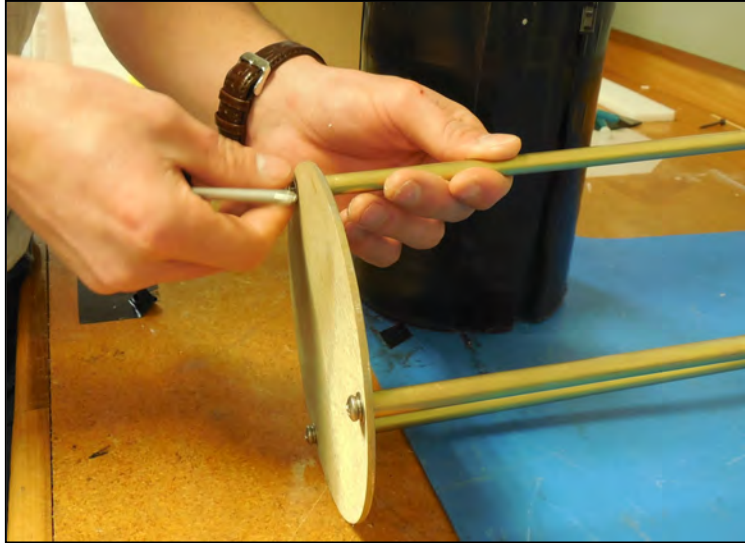
Figure A.1.3-4: Removing Battery Housing End Plate
