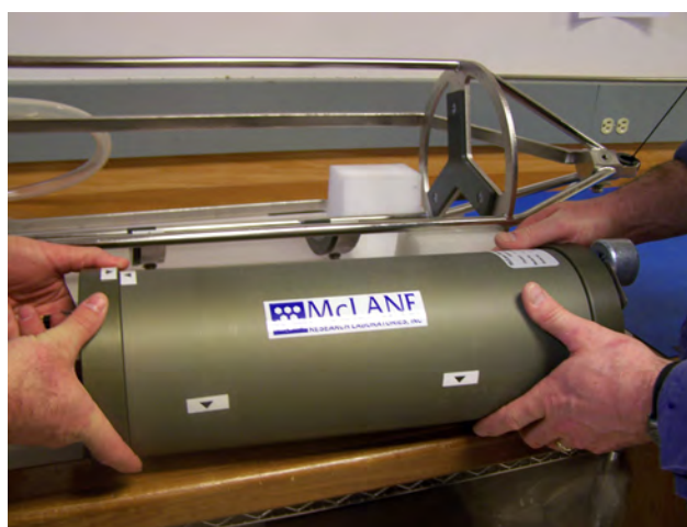
Figure A.3-12: Removing Controller Housing
