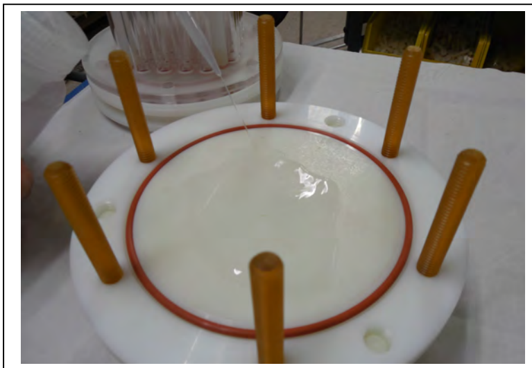
Figure 6-15: Flood the Filter Holder Bottom Plate
