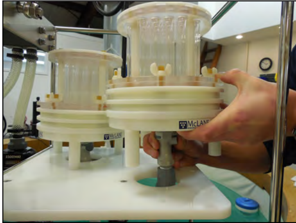
Figure A.1.2-5: Securing Filter Holder to Quick Disconnect
