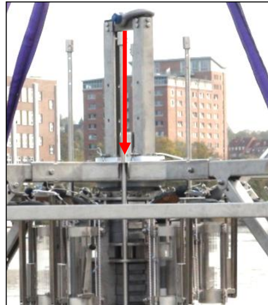
Figure 32: Lower the head in order to flush the damping tube
