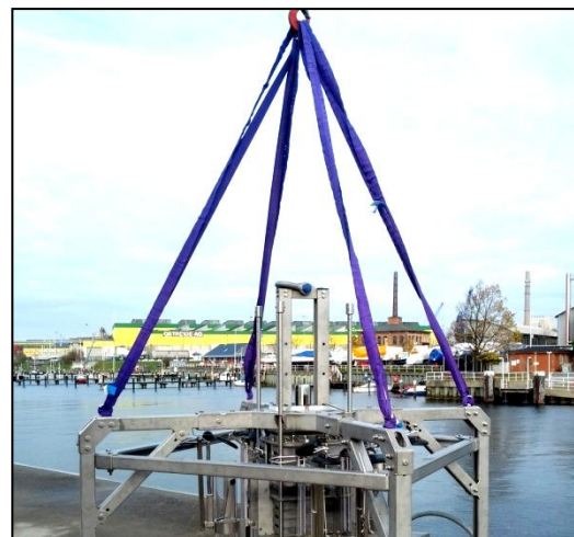
Figure 6: Multi Corer hooked on to the 4 lashing points
