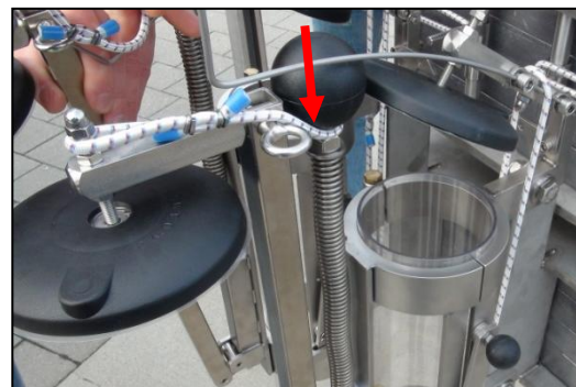
Figure 13: Fastening the lower locking arms
