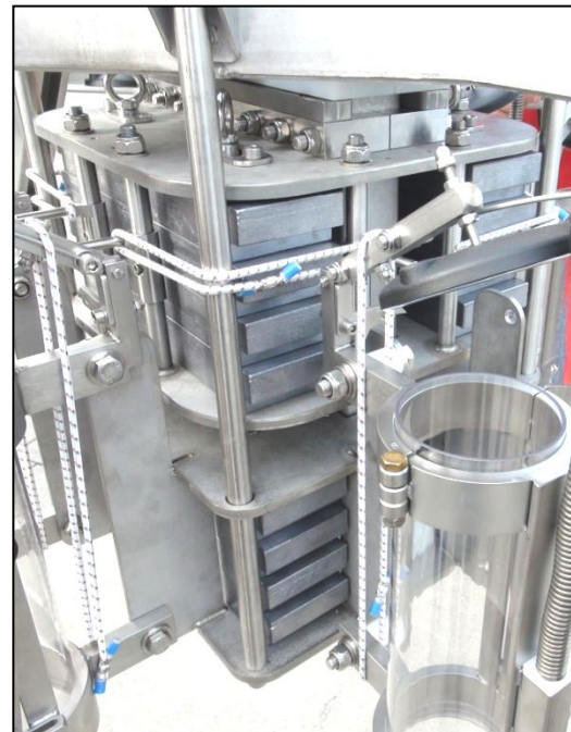
Figure 19: Replacing lead bricks
