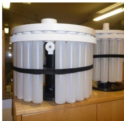
SUPPORT FOR RECOVERY SAMPLES (Can be used for 12 or 24 samples carousel and 250 or 500ml bottles)
