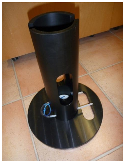
SUPPORT FOR RECOVERY SAMPLES (Can be used for 12 or 24 samples carousel and 250 or 500ml bottles)
