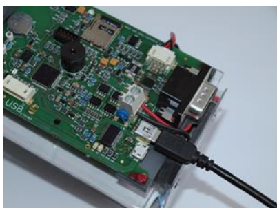
Internal communications USB connection cable / Communication interne Câble de connexion USB
