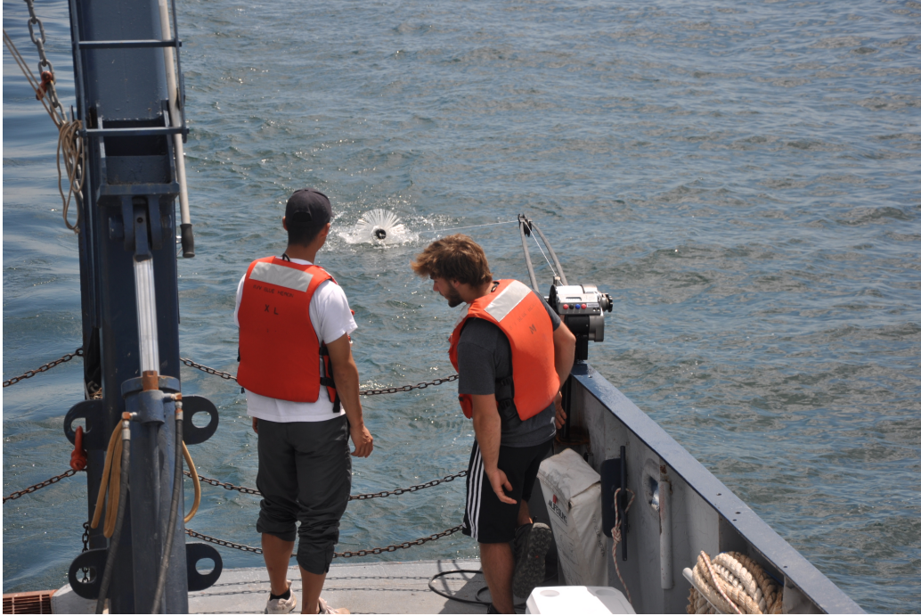
Figure 4: An LP S-1200 Electric Reel mounted for Tow-yo operations. The VMP is being towed on the surface while the vessel is underway. Photo credit: Dan Titze
