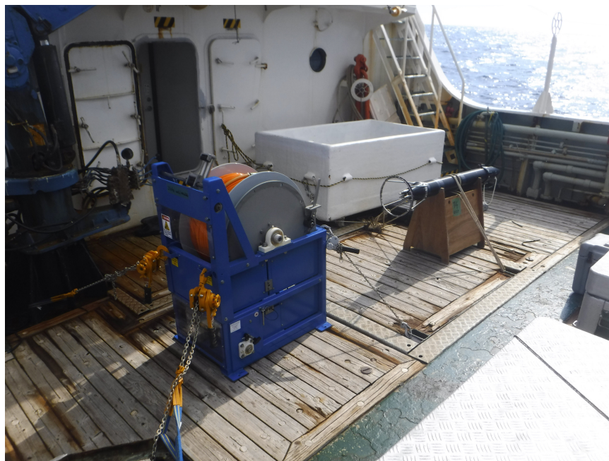
Figure 2: An A.G.O. Environmental CSW-7 Conventional Winch installed amidships to deploy a VMP-500-RT
