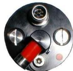
The magnetic power ON/OFF switch is not used and is bypassed when the probe is used with telemetry (please remove the internal batteries, if any, before operating the probe through the telemetry system).
