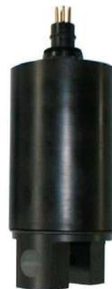
The calibration procedure is the same described for the turbidity meter. The only differences are the measuring scales, which in the case of the fluorometer are: 5, 15, 50 and 160 µg/l.
