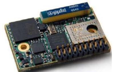
IDRONAUT Windows programs like REDAS-5 and ITERM flawlessly operate the OCEAN SEVEN 310 through the Wireless Module as if it were connected through an RS232 cable.
