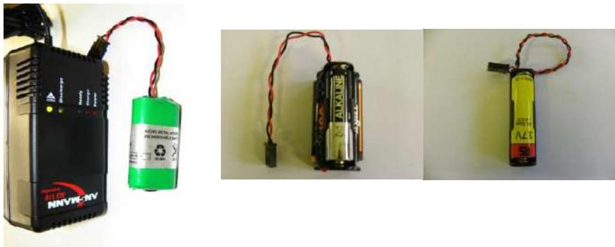
OCEAN SEVEN 310 is shipped without batteries installed. Please be aware that **it is not possible to recharge the battery pack when it is installed inside the probe**
