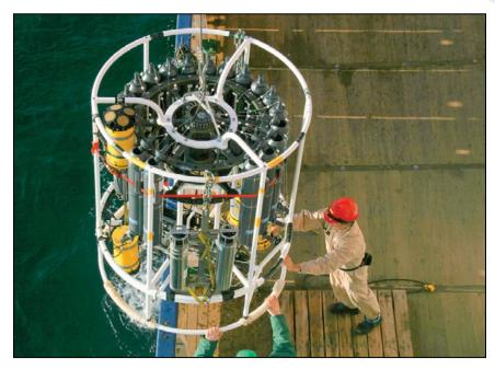
Dual Teledyne RDI ADCPs (colored yellow for high-pressure rating) are attached to a hydrographic package.
