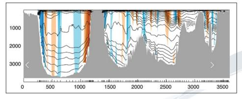
Strong currents were seen at various levels. In particular, the LADCP data showed a high-speed core near the deep-sea floor. Its waters had originated in the Nordic Seas.
