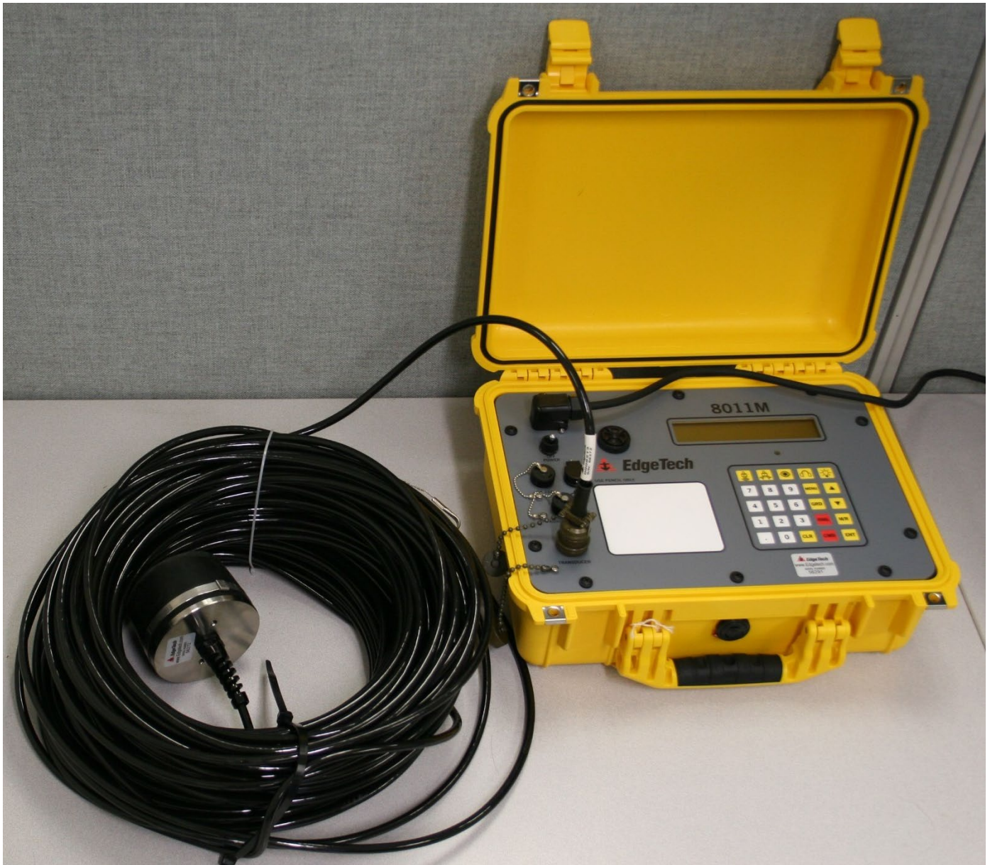
Figure 3-2: 8012M Transducer Installed into the 8011M Deck Unit
