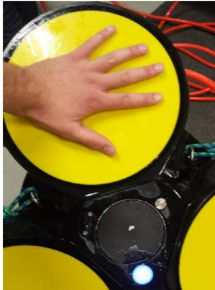
Figure 7. Example of an amplitude test. Rub or tap the transducer with your hand
