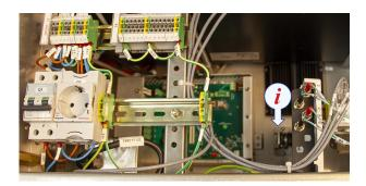
7 Slide the power unit to the left and pull out the power module.
