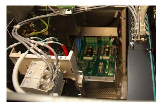
Make sure the cables are tucked in at the sides, so they won't be damaged when the module is removed.
