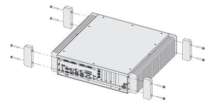
2 Fasten the rack adapter parts on each side with 12 M4 pan headed screws.
