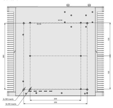
The computer has two different hole patterns included. Use four M6 or six M4 fasteners to mount the computer.
