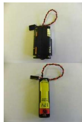
**INSTALLING TWO 3.6V LITHIUM BATTERY IN THE DOUBLE ALKALINE BATTERY HOLDER AND CONNECTING IT TO THE OS304*Plus* TOP COVER WILL CAUSE A PERMANENT DAMAGE TO THE OS304*Plus* CTD ELECTRONICS.**
